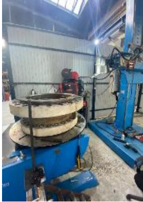
Inconel Overlay Welding Station
