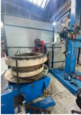
Inconel Overlay Welding Station
